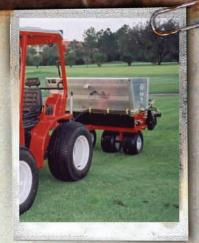
The economical 10 series top dressers are ideal for use with low horse power compact tractors and can be either mounted on a 3-point linkage or trailed on four pivoting high flotation wheels to minimize ground pressure. Both models use the tractor hydraulics to power the guided belt and brush applicator. The Rink delivery system ensures an even spread with all spreading materials, even wet sand.
